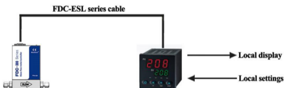
Figure 5 Connected to the Flow Control Unit
