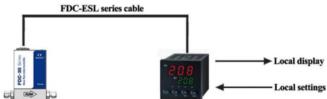
Figure 5 Connected to the Flow Control Unit
